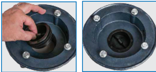
Remove drain barrel/strainer from the drain base and gently push waterless trap seal into the hub of the drain. Replace the drain barrel/strainer.
