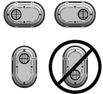
Figure 6b – Approved Installation Orientation
