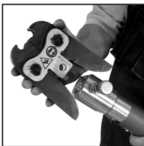
Figure 7: Placement of adapter jaw into the tool
