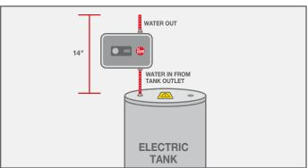
Once both water lines are fastened and secured, you MUST RUN WATER through the unit for at least 2 to 3 minutes to flush any air pockets (purging) in the lines and make sure there are no leaks. It is recommended that all faucets, showers etc. be run. Failure to follow this step can cause permanent damage to the unit. This procedure MUST be performed before any electrical power is turned on.
