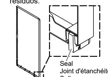
**16** Install the end walls. Engage the end wall pins in the back wall slots.
