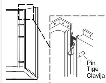
**17** The front edges should be flush, with no more than a 1/32" (1 mm) gap.
