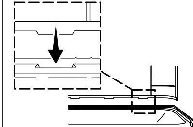
**13** Measure, mark, and drill the faucet holes in the drain end wall.
