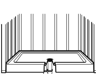
**10 Custom Walls:** Cut the finished wall as shown. Leave the weep channel open.
