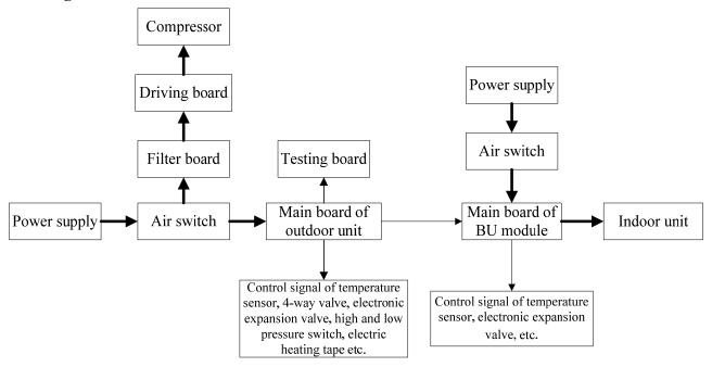
(The thick line represents power line while thin line represents the control line.)
