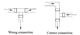
Confluence toward the horizontal pipe shall be best from the upper. Back flow is easy to occur if from the lengthwise direction.
