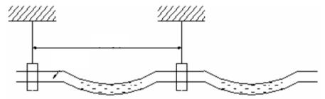
15) If the air flow of indoor unit is high, this might cause negative pressure and result in return suction of outdoor air. Therefore, U-type water trap shall be designed on the drainage side of each indoor unit.
