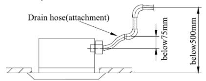
• Please install the drain hose according to the following process if several drain hoses join together.
