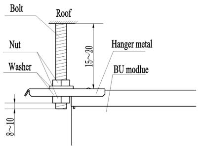
5) Adjusting the nuts position, so that the BU module should be level in front/back and left/right.
