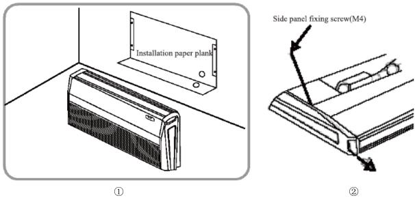
2) Remove the return grill, the side panel and the hanger bracket from the indoor unit as per procedure bellow.
