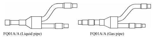
2) Y-type branch pipe is equipped with auxiliary tubes to adjust the diameter of different pipes. If the dimension of the pipe selected is different from the dimension of branch pipe joint, Cut the copper tube in the middle with tube cutter and clear up burrs. Please do that as following figure.
