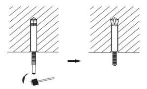
4) Fix the modules securely with the hanger bolts. You can get the M10 or M8 hanger bolts, nuts and washers from the market.
