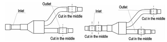
3) Y-type branch pipe must be installed in vertical or horizontal direction. In the inlet of the branch pipe, keep at least 500mm straight pipe.
