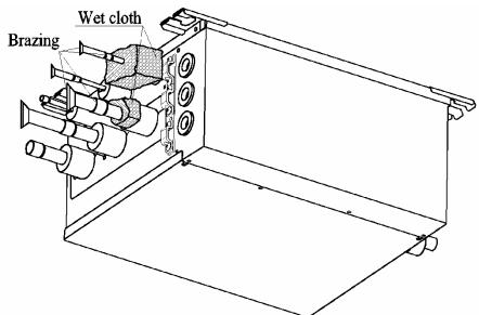
4 After brazing, use wet cloths to cool off the pipes to be brazed sufficient.
