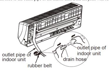
2) Put the drain hose into insulating tube.
